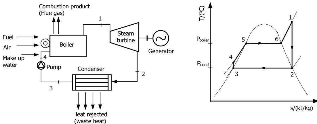
**Fig 1** – Schematic diagram of hardware arrangement of a steam power plant (left) and Rankine cycle (with superheat) on temperature - entropy (T-s) plane (right)
