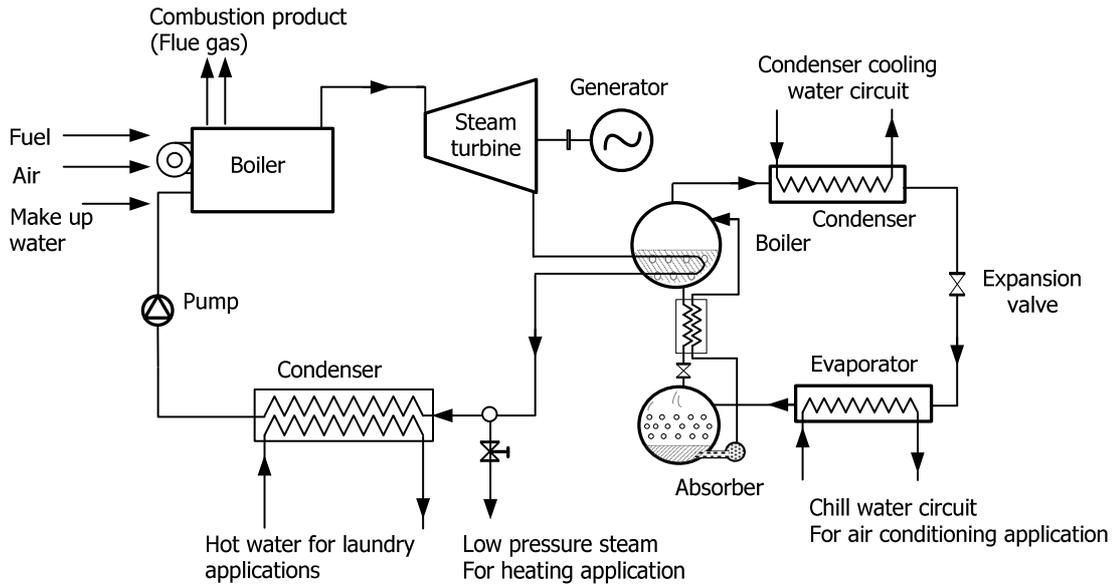
b) Trigeneration system – Power, cooling and heat
