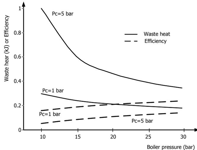
**Fig 2** - Effect of main operating pressures on the heat output and efficiency of steam power plants (generated using REFPROP [3] based on Rankine cycle with superheat)
