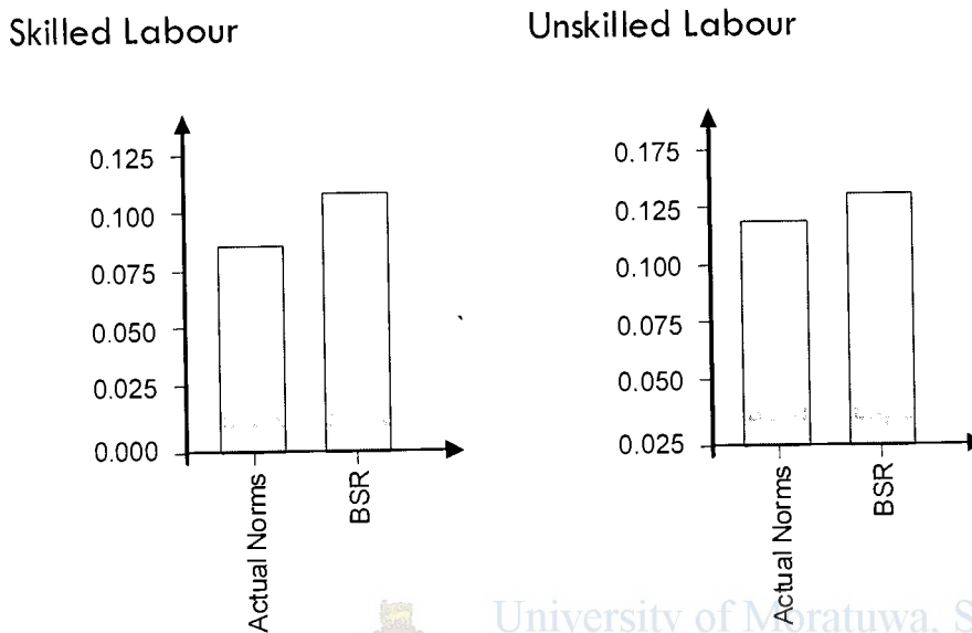
Figure 5.6: Comparison between labour consumption on internal plastering works and BSR Standard
