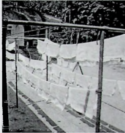
Fig 4: Sheets are kept under sunlight for dripping of water
