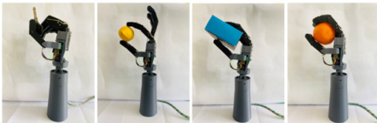
Figure 2: An array of grasping patterns produced by the device
