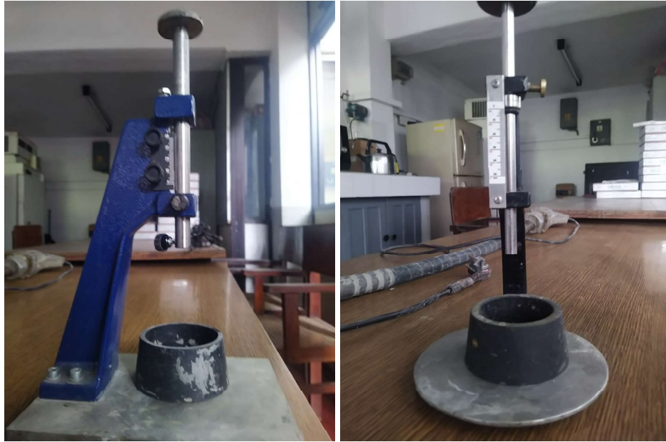
(a) Vicat plunger to determine consistency (b) Vicat plunger to determine setting time
