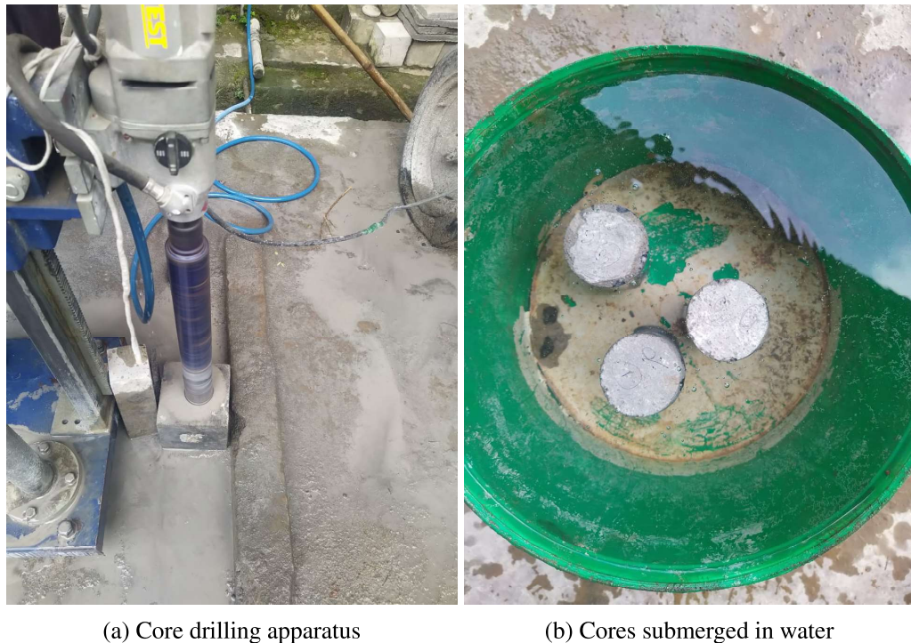
Fig. 3.11: Water absorption test
