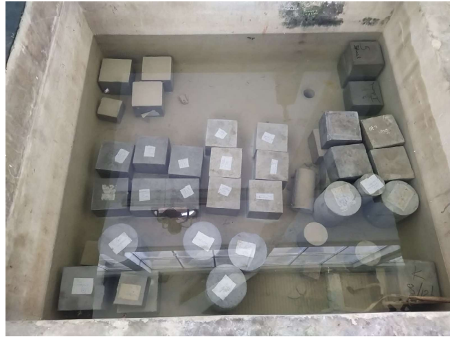
(b) Curing tank
