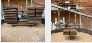
The experimental setup was loaded, and settlements were measured
