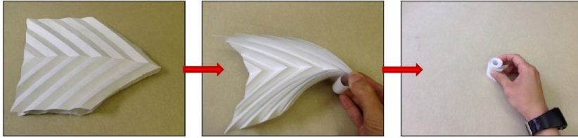
Curved beech leaf pattern inspired membrane antenna prototype
