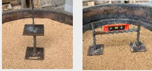
Two prototype footings
