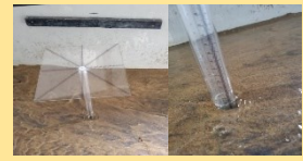
Model of bridge pier (Acrylic Plastic)
