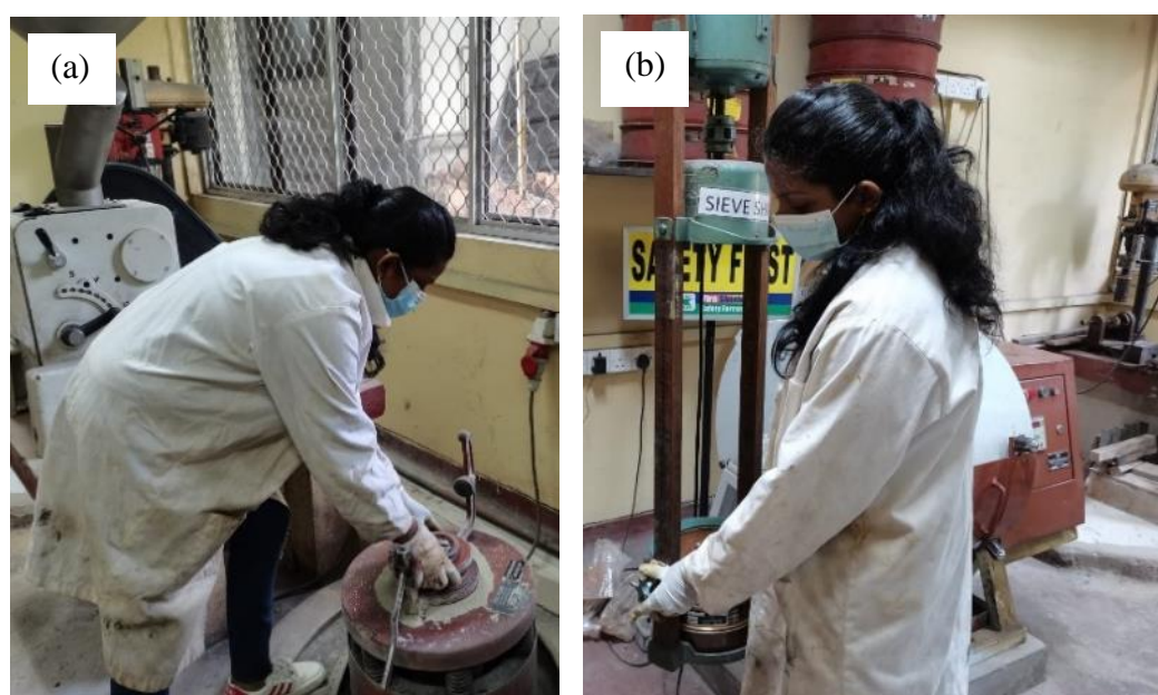
Figure 3.18: (a) Powdering rock/soil/sediment samples using the laboratory Tema mill; (b) Sieving through 63 \mu\text{m} sieve to reduce the particles size in samples
