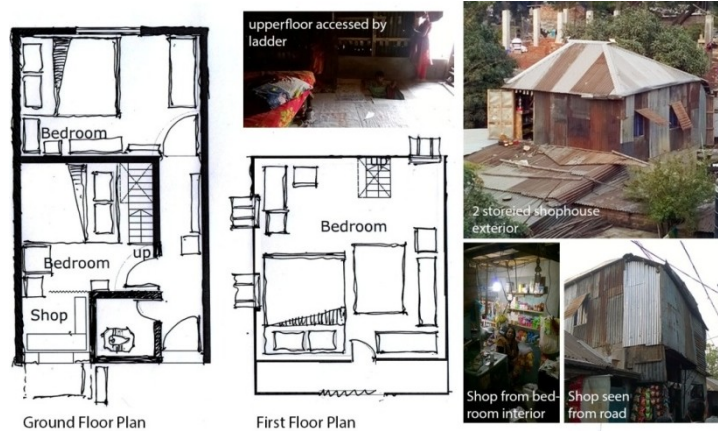
Fig 09: Plan and section of a spontaneously developed Semi-pucca House Source: Authors
