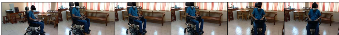
Fig. 2. The sequence of diagrams illustrates how a user can smoothly control the wheelchair with the developed layered hardware and software module. The sequence begins from the leftmost image which depicts the user moving in a straight course and changing his trajectory by turning the Wheelchair by 90°. The generated trajectory is a curved path since the user selects both move forward and turn functions simultaneously.
