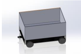
Fig. 1. Design of Tigger part of the AGV
