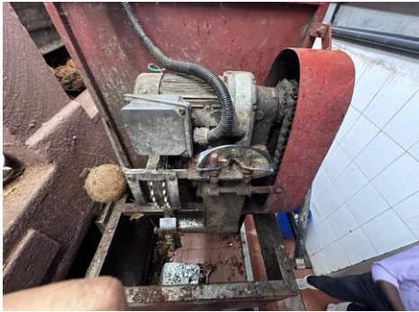
Fig. 4: Existing deshelling machine
