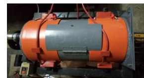
Fig. 2. Container with heater pads
