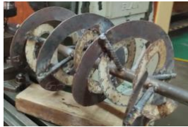
Fig. 5. Double ribbon mixture
