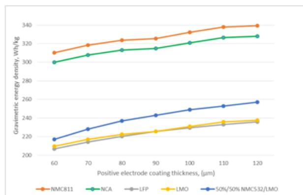
Figure 5: The volumetric energy density comparison for five positive electrode materials under variable electrode coating thickness
