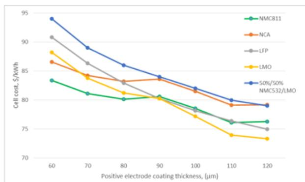
Figure 4: Cell cost comparison for five positive electrode materials under variable electrode coating thickness
