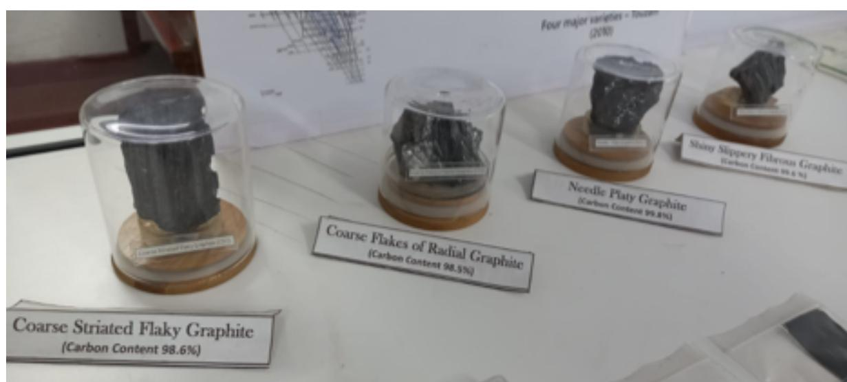
Figure 3: Types of Sri Lankan vein graphite
