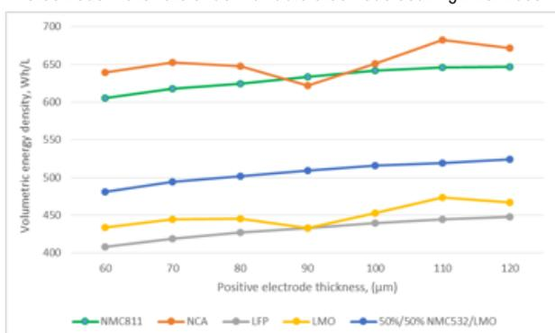
Figure 6: The gravimetric energy density comparison for five positive electrode materials under variable electrode coating thickness
