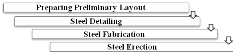
Figure 1: Steel building frame construction process Source: (Mehta, Scarborough & Armpriest, 2010)
