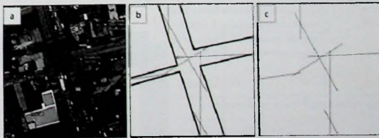
Figure 6: Preparation of axial lines Notes: a. Google image, b. axial line preparation, c. axial map Source: Author constructed
