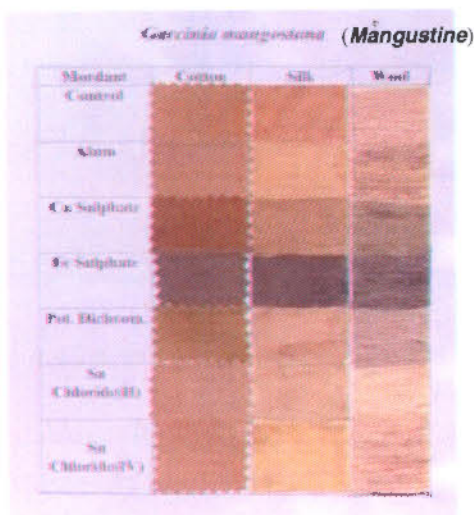
Figure 4.42 Fabric samples dyed with methanolic extract of G. mangostana with different mordants
