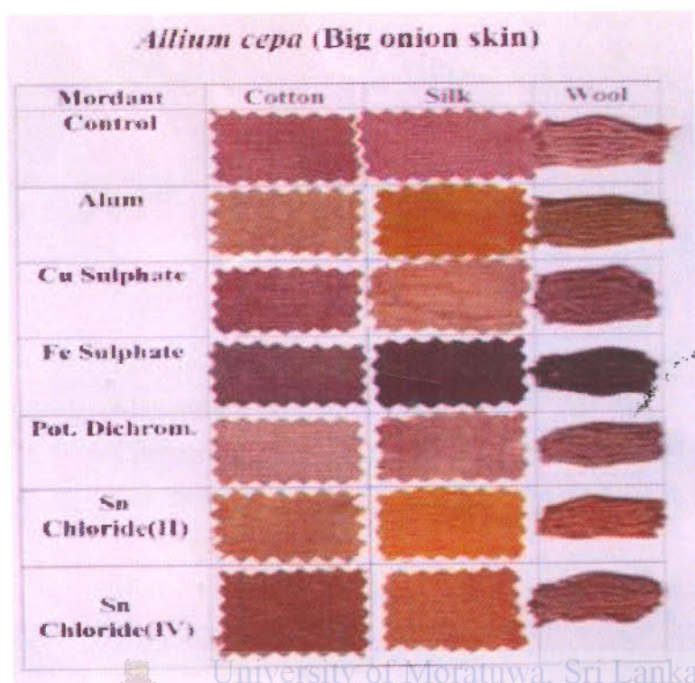
Figure 4.36 Fabric samples dyed with methanolic extract of A. cepa with different mordants.
