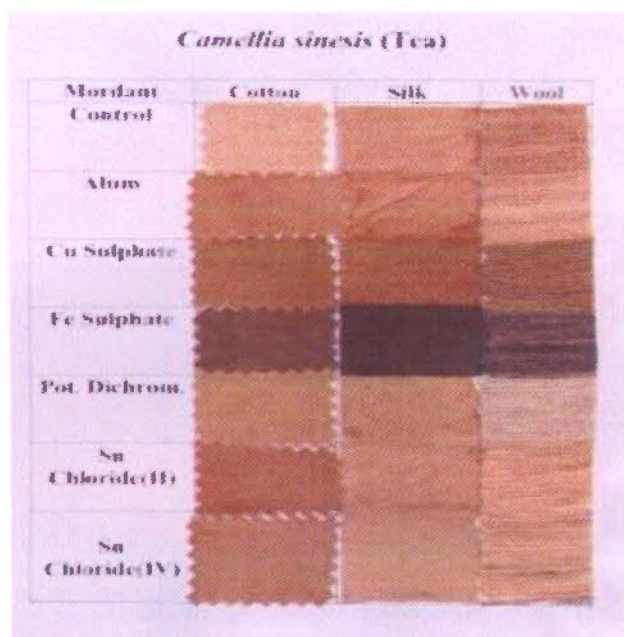
Figure 4.54 Fabric samples dyed with methanolic extract of C. sinensis with different mordants.
