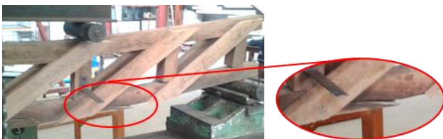
Figure 8: Flexural splitting in Pratt
