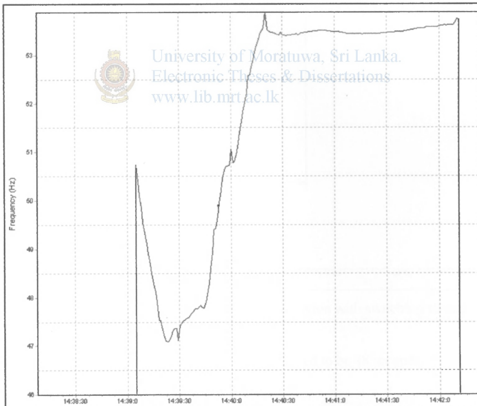
Figure 7.2 – Frequency Vs Time during synchronization with switching strategy I.
