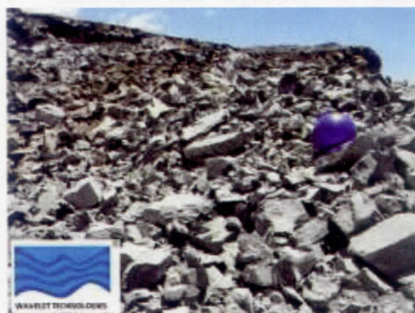
Figure 5(a) - Input image of blast muck pile from mobile camera
