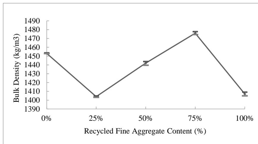
Figure 3: Bulk Density (kg/m<sup>3</sup>) vs. RFA Content (%)
