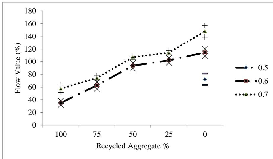
Figure 5: Flow Value (%) vs. RFA Content (%)
