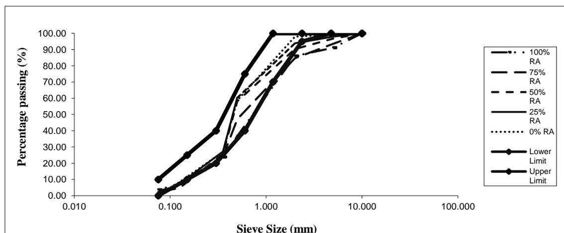
Figure 1: Percentage Passing (%) vs. Sieve Size (mm)
