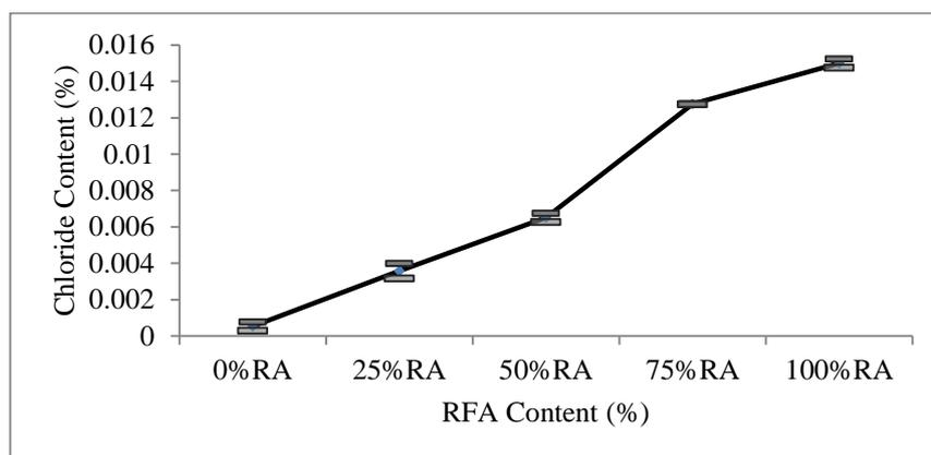
Figure 4: Chloride Content (%) vs. RFA Content (%)
