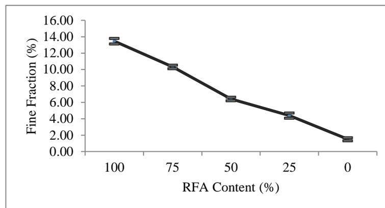
Figure 2: Fine Fraction (%) vs. RFA Content (%)
