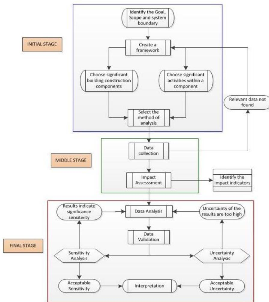
Figure 4: General Methodology for Carrying Out LCA in Buildings
