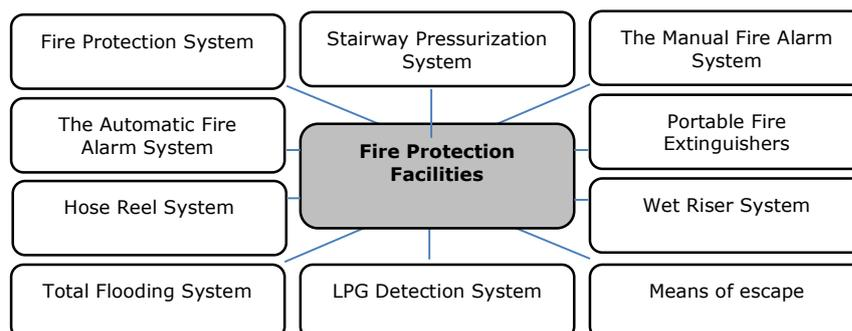
Figure 1: Essential Fire Protection Facilities
