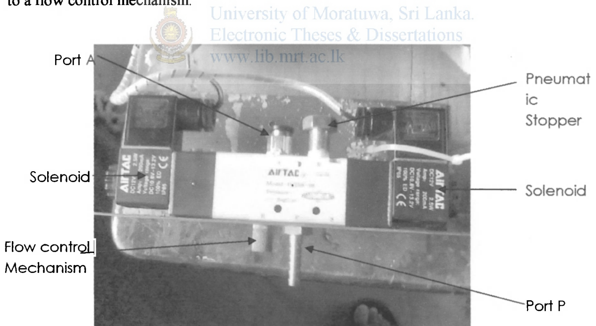
Figure 4.4: Port Allocation of the Valve
