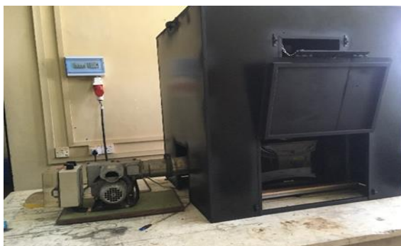
Figure 3.1 Microwave assisted air dryer designed and fabricated for the experiments
