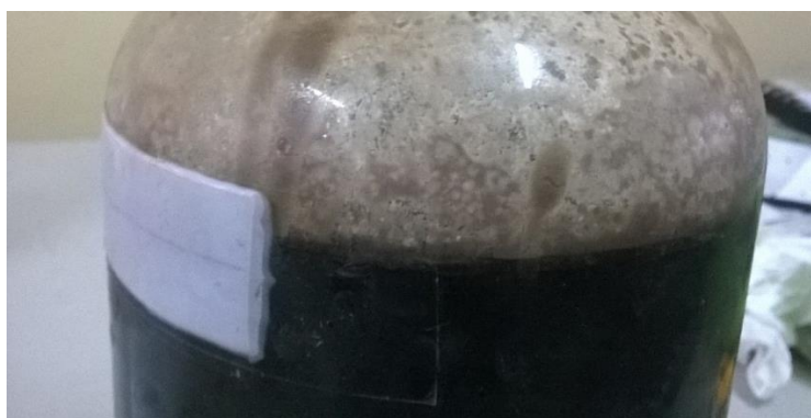
Figure 4.64: Elemental sulfur formed on the walls of the head space of the reactor
