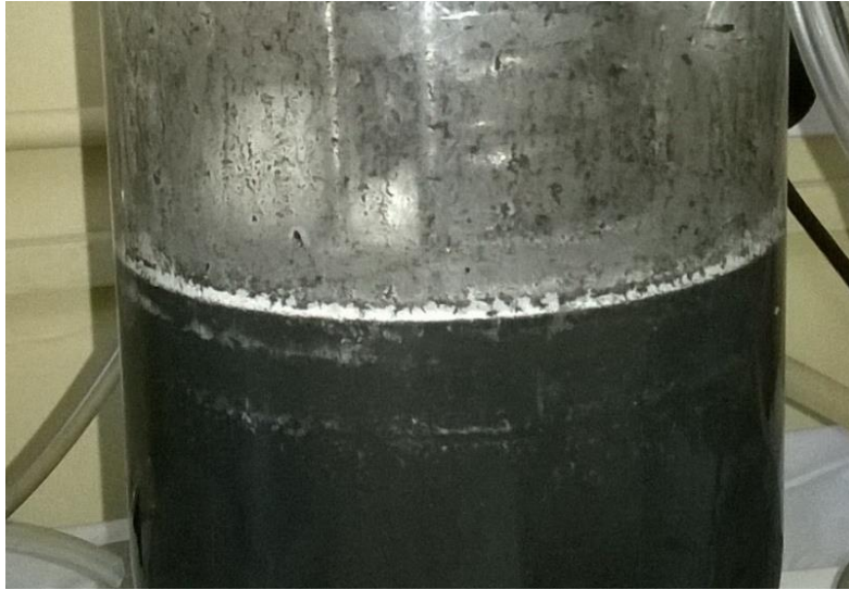
Figure 4.79: Elemental sulfur formed on the wall of the head space and the gas-bulk liquid inter-phase
