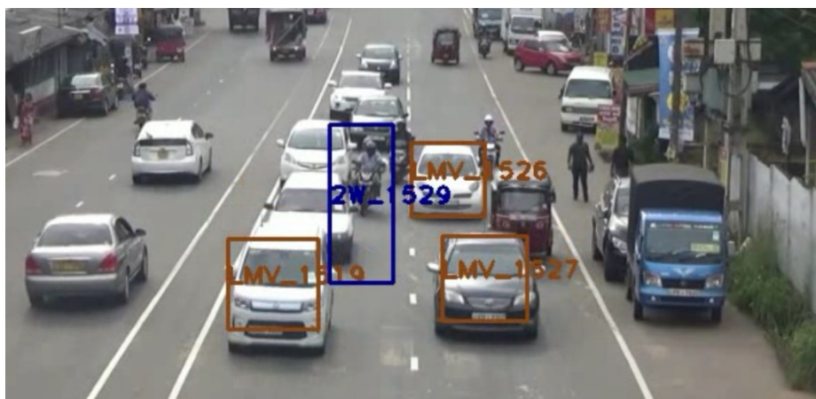
Figure 3.10: TRAZER video detection – A4 highway, Pannipitiya
