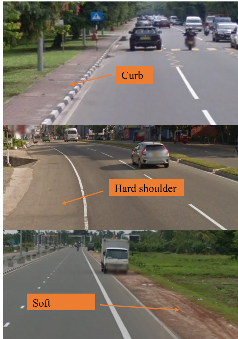
Figure 4.4: Shoulder types available on multi-lane roads
