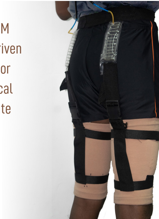
Figure 1: Sit-to-stand transition assist exosuit
