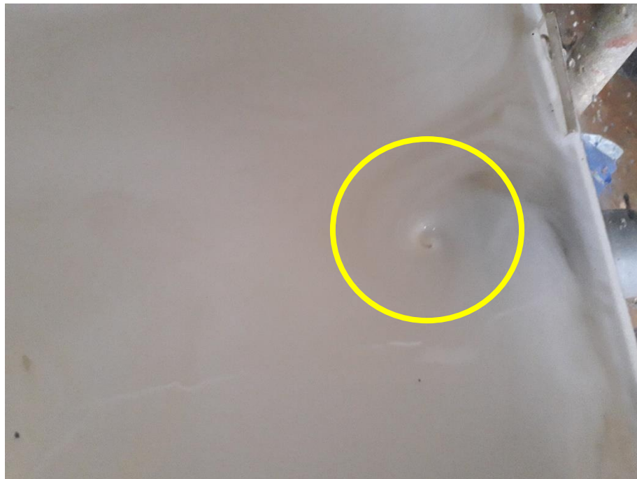
Figure 3- 3: Air core type 06 Vortex formed in the physical model
