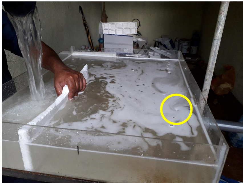
Figure 3- 1: Physical Model operating with a dye to track vortex formation
