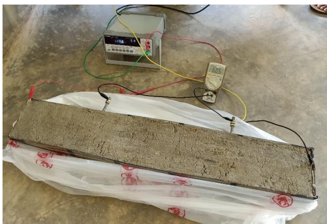
Figure 5.20: Soil box testing for location 2
