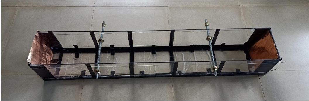
Figure 5.5: Created Soil box for soil resistivity measurement
