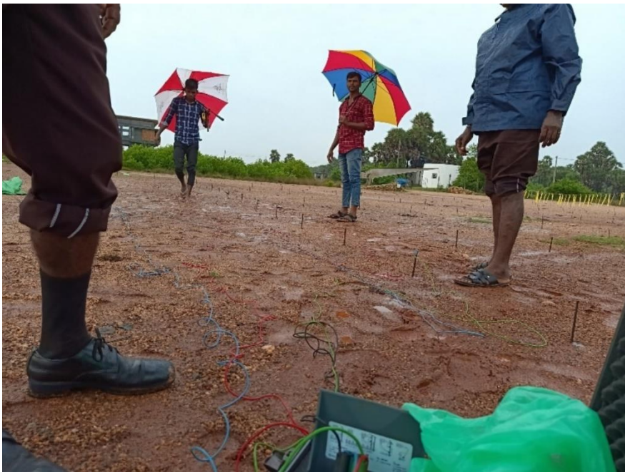
Figure 5.18: Earth Resistivity probe arrangement – Location 2
