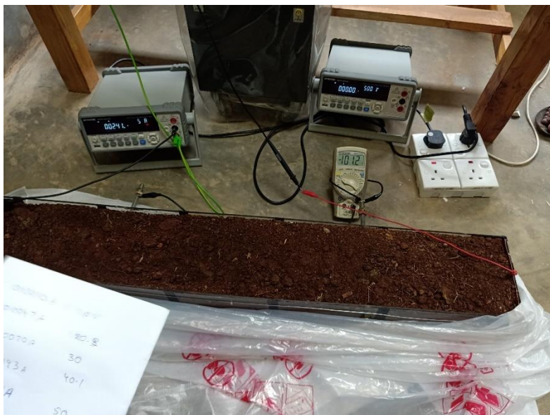
Figure 5.12: Soil box testing for location 1
