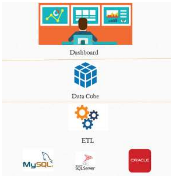
Figure 1.1 : OLAP Design with SQL Data Sources Separating each Layer
