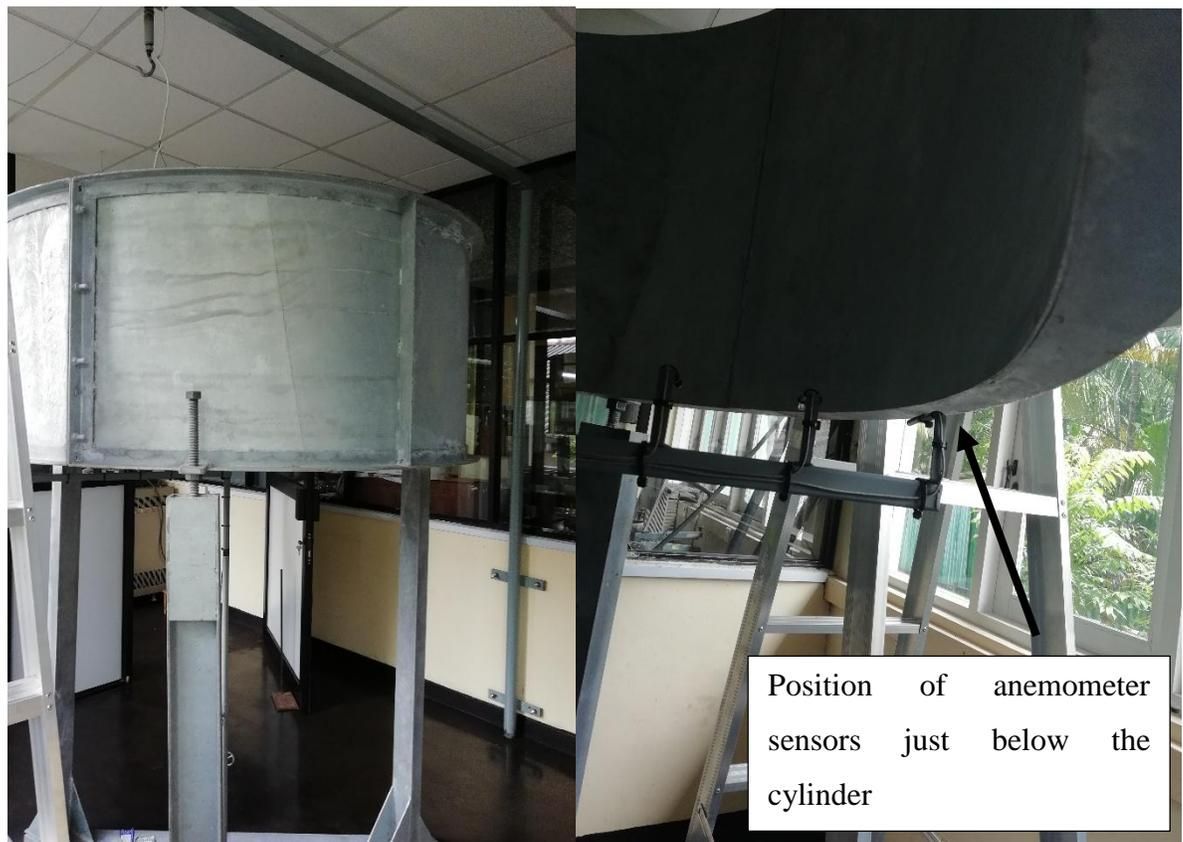
Figure 3.2 – Test chamber containing the cylinder and the placement of anemometer sensors
