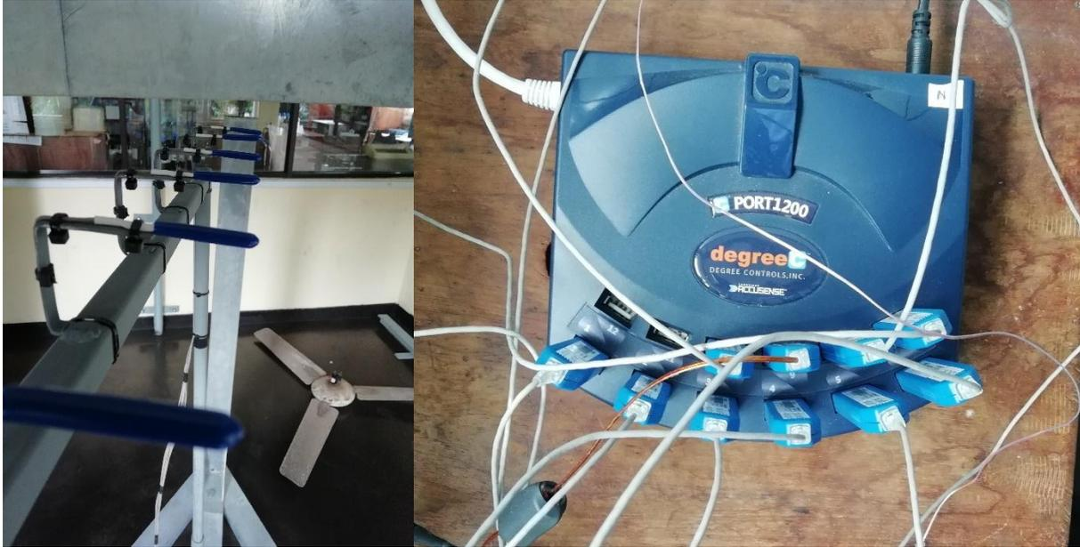
Figure 3.3 - Anemometers probe and DAQ card
