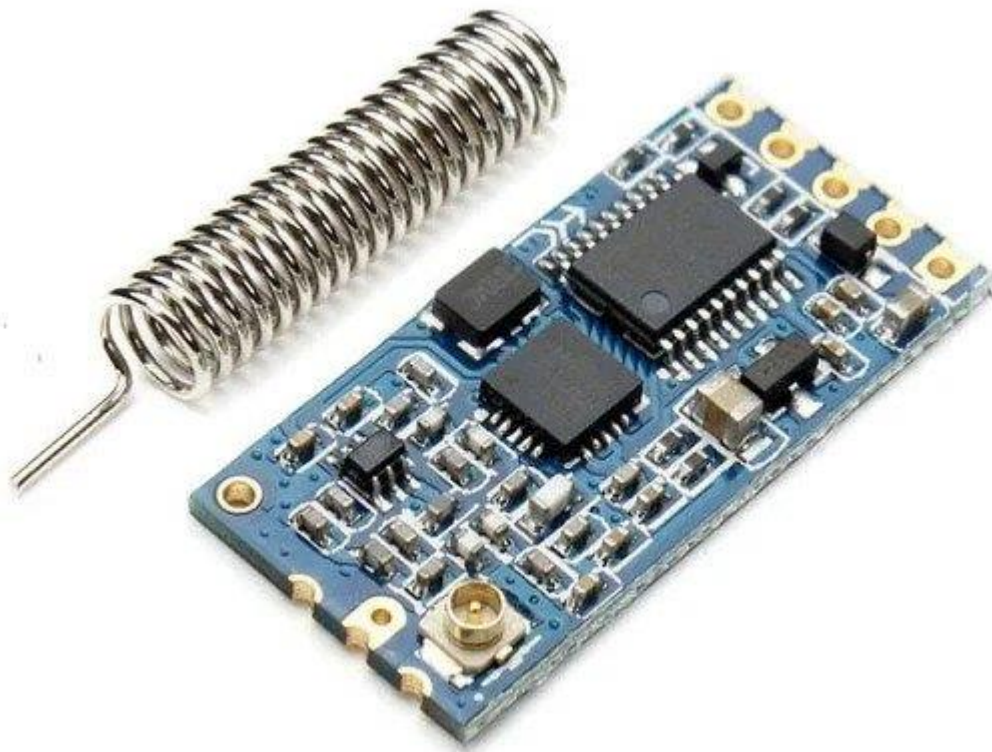
Figure 3. 2: HC-12 Wireless Serial Port Communication Module
