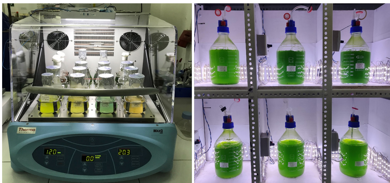
Figure 2: Microalgae cultures maintained in incubators (left) and cultivated in lab-scale photobioreactors (right) at the Department of Chemical and Process Engineering, University of Moratuwa
