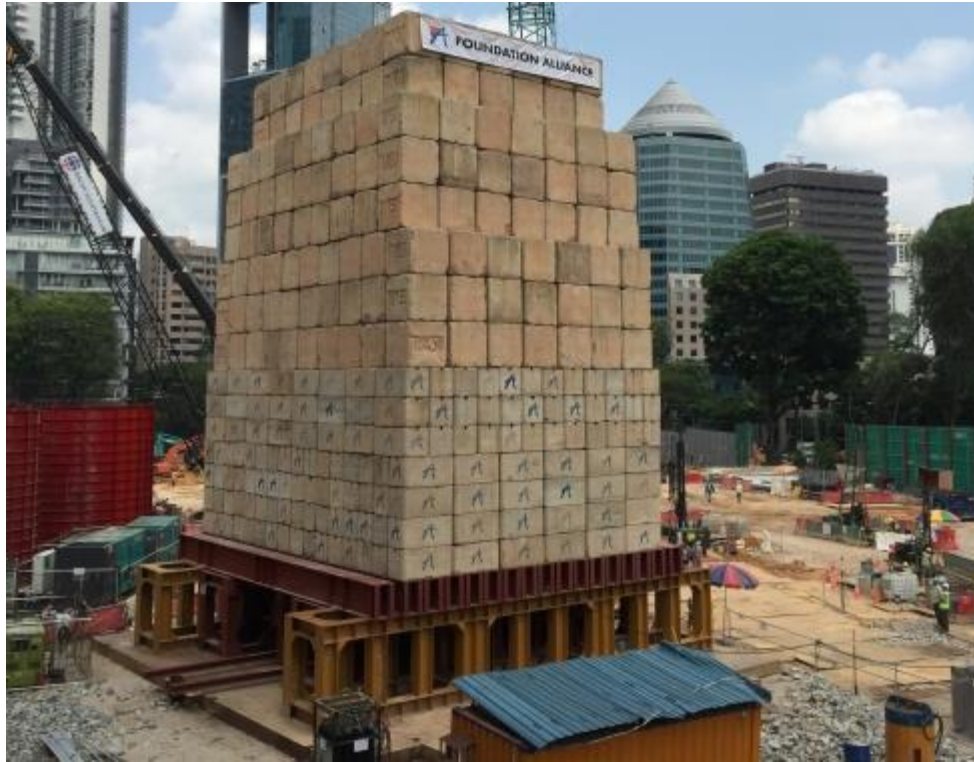
Figure 12. MLT test arrangement with loading blocks
