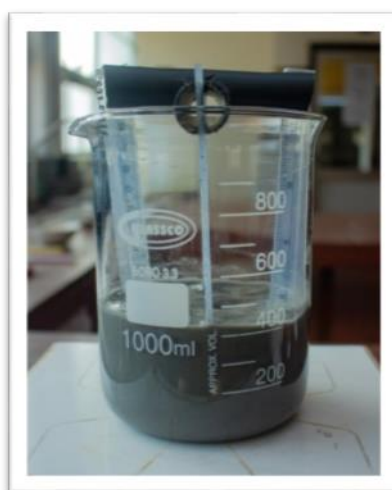
Figure 3.2: Laboratory mixer for calcium extraction from fly ash
