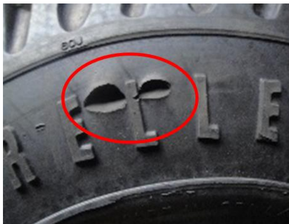
Figure 40: Surface defects on side wall
