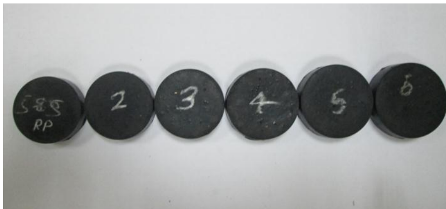
Figure 16: Standard test sample for tensile test
