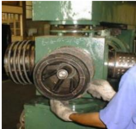
Figure 18: Use of expandable drum for green tire building
