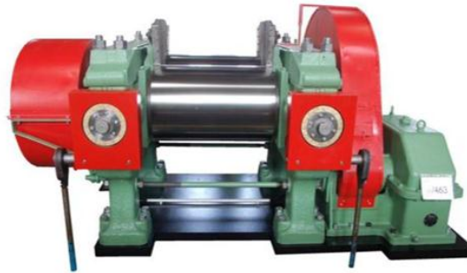
Figure 9: Industrial two roll mill
