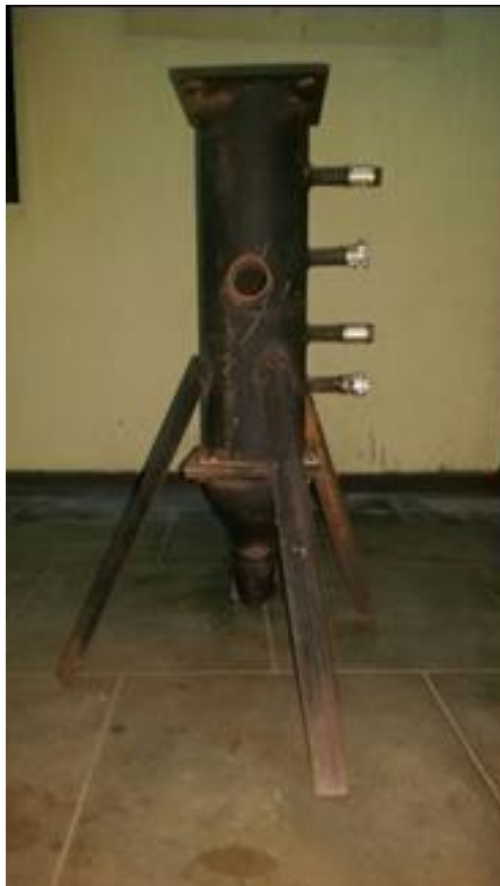
Figure 4.1- Fluidized bed combustor apparatus
