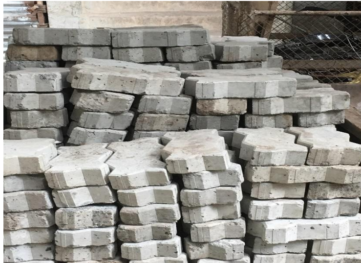
Figure 4.8 : Paving blocks from concrete waste in Case B
