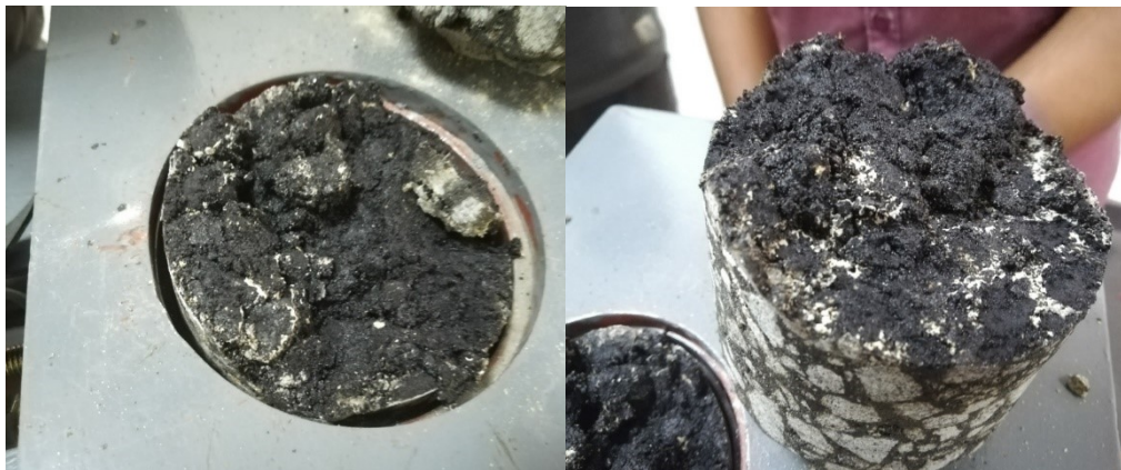
Figure 56. Failure plane of the core sample (a) above the interface (b) below the interface
