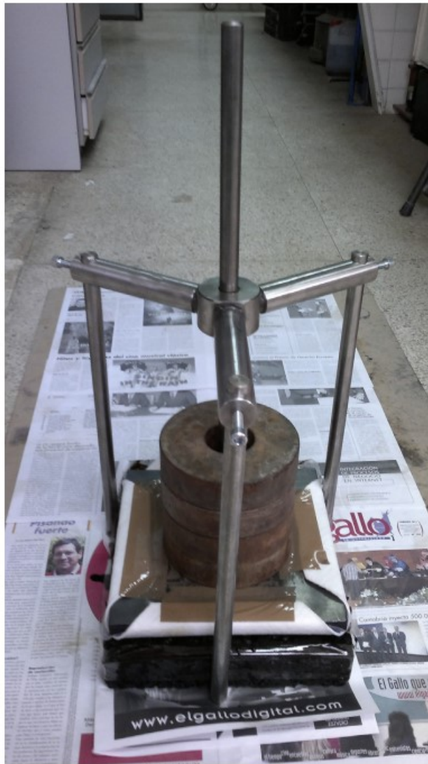
Figure 7. Absorbed emulsion content test
