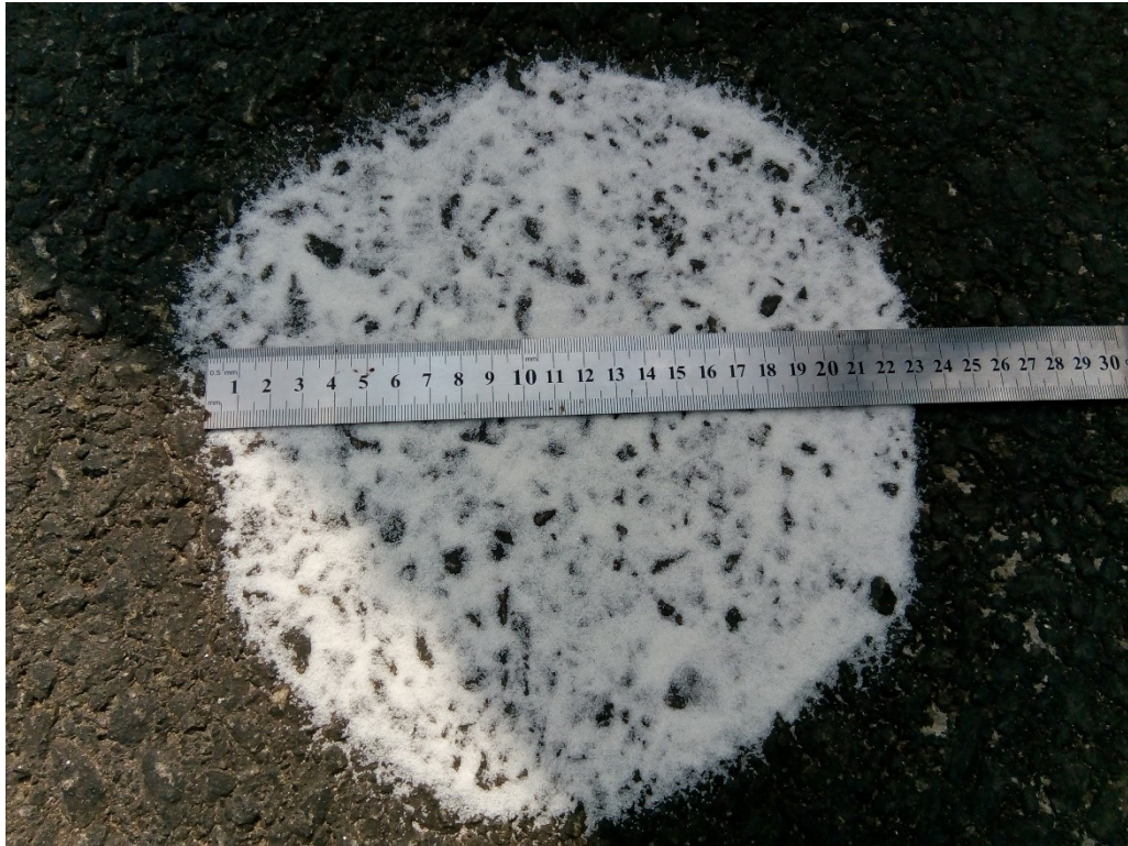
Figure 15. Sand patch test
