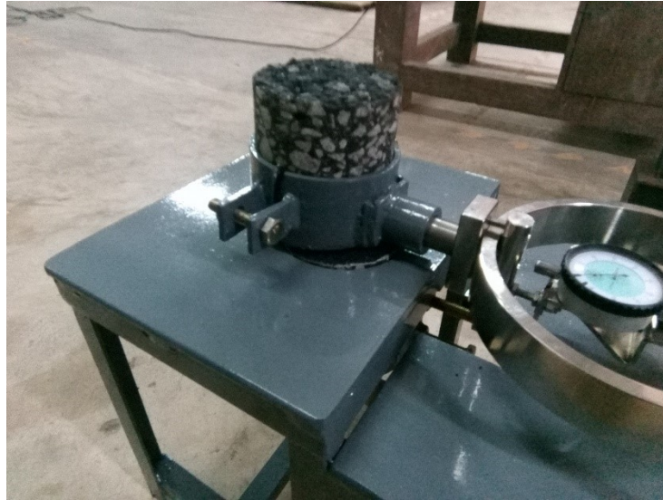
Figure 35. Core sample at the failed moment
