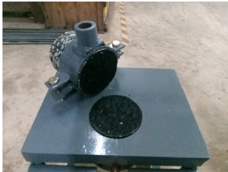
Figure 36. Failed core sample
