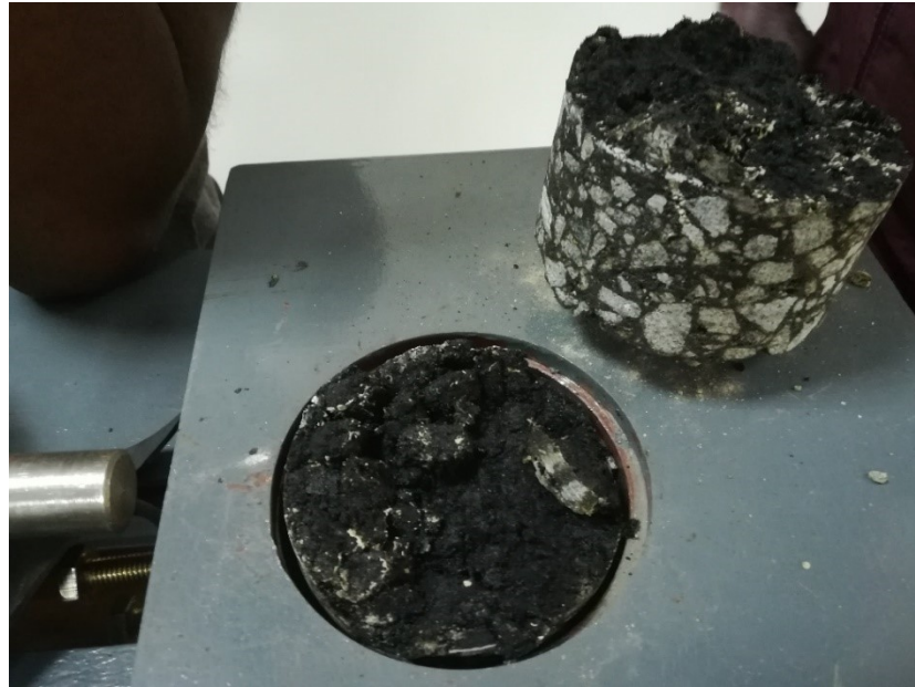
Figure 55. Core sample, not failed at bond
