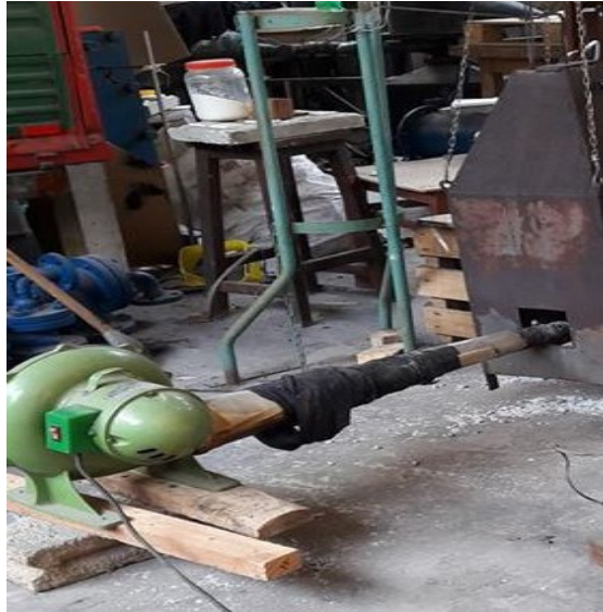
Figure 3-5 : Picture of the Primary air Supply Blower
