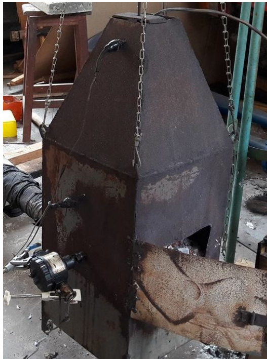
Figure 3-2 : Picture of the Thermocouples with Reactor
