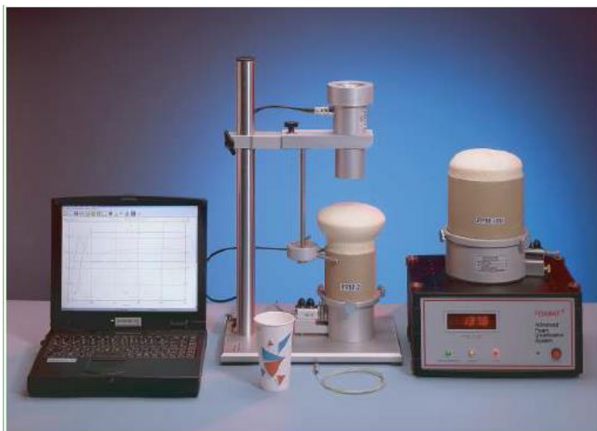
Figure 3.8: Basic parts of the FOMAT equipment
