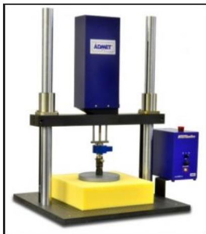
Figure 3.7: Foam compression device
