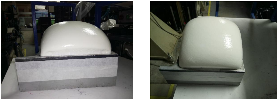
Figure 3.2: Polyurethane foam produced in the Standard box mold
