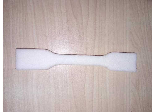
Figure 3.12 test specimen for Elongation test
