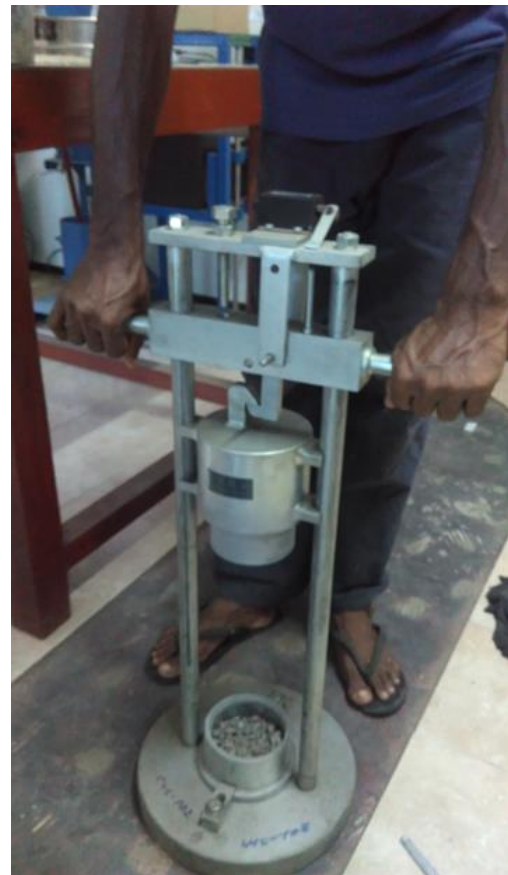
Figure 3.4: Aggregate Impact Value test
