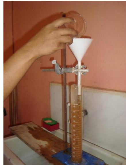
Figure 3.4 - Experimental Setup of Sludge Cohesion Test
