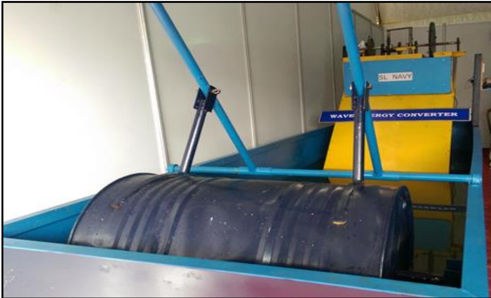
Figure 4.23: Wave making facility in Final Prototype model of Oscillating Power Buoy operated Rack & Pinion Power Take-off WEC
