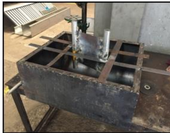
Figure 4.1: Fabrication of the buoy
