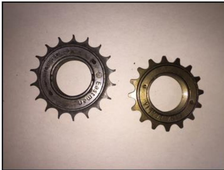
Figure 4.7: Gear wheels used for the Drive shaft
