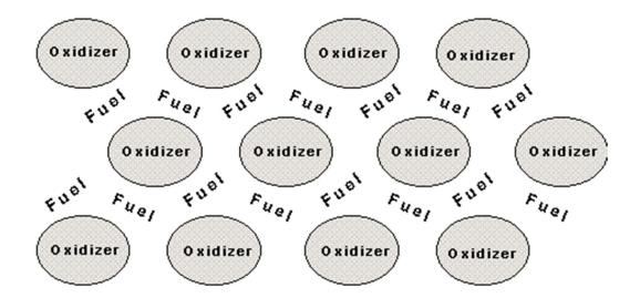
Figure-4: Schematic of Water-in-oil emulsion.
