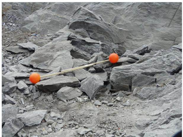
*Figure-21.5*: Location - 06, Blast -05(Scale: Ball diameter is 20.32 cm)
