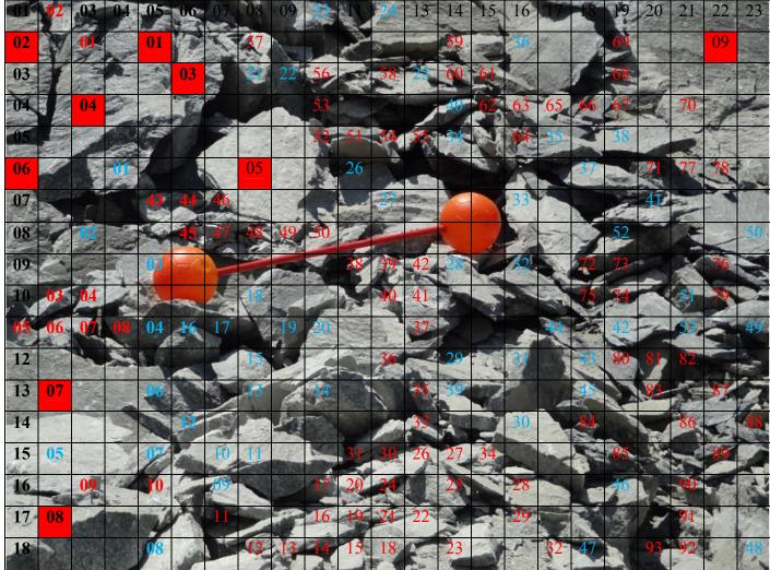
*Figure-19-5.1*: Location - 04, Blast -05 -Fragmentation Analysis (Scale : Ball diameter is 20.32 cm)
