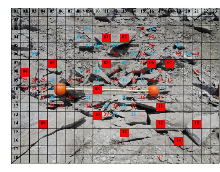
*Figure-21.3.1*: Location - 06, Blast -03, Fragmentation analysis (Scale : Ball diameter is 20.32 cm)
