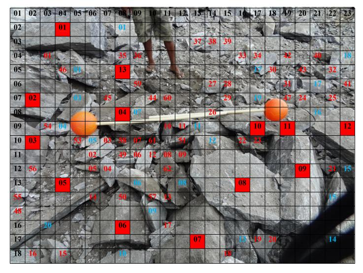
*Figure-21.4.1*: Location - 06, Blast -04, Fragmentation analysis (Scale : Ball diameter is 20.32 cm)
