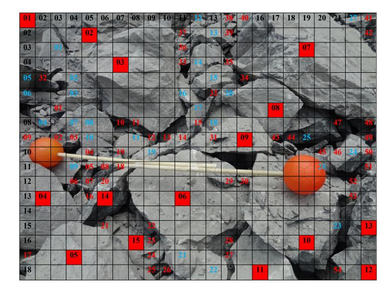
*Figure-20-3.1*: Location -05, Blast -03- Fragmentation Analysis (Scale: Ball diameter is 20.32 cm)
