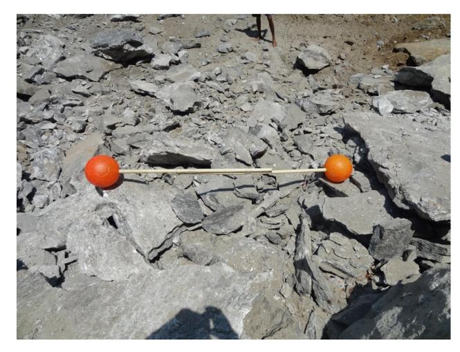
Figure-16.3 :Location -01, Blast -03- (Scale: Ball Diameter is 20.32cm)
