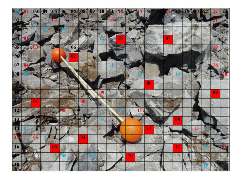
*Figure-17.2.1*: Location - 02, Blast -02-Fragmentation Analysis (Scale : Ball diameter is 20.32 cm)
