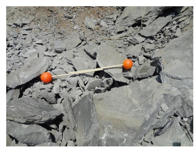
Figure-16.6 :Location -01, Blast -06 - (Scale: Ball Diameter is 20.32cm)
