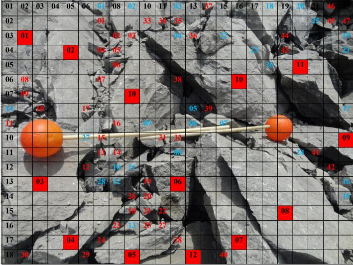
*Figure-20.2.1*: Location -05, Blast -02 -Fragmentation Analysis (Scale : Ball diameter is 20.32 cm)
