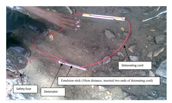
Figure-7.1: Sketch for the preparation to test the VOD by Dautriche method
