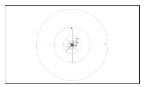
*Figure - 2.* Schematic illustration of tension crack length and density around single shot blast hole. [Source - Internet - TORBICA,S.,LAPCEVIC,V.Rock breakage by explosives. European International Journal of Science and Technology, p. 96-104, 2014.]
