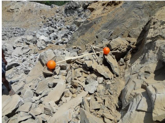
Figure-18-2: Location - 03, Blast -02- (Scale: Ball diameter is 20.32 cm)
