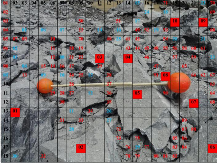
*Figure-20-5.1*: Location -05, Blast -05 - Fragmentation Analysis (Scale : Ball diameter is 20.32 cm)
