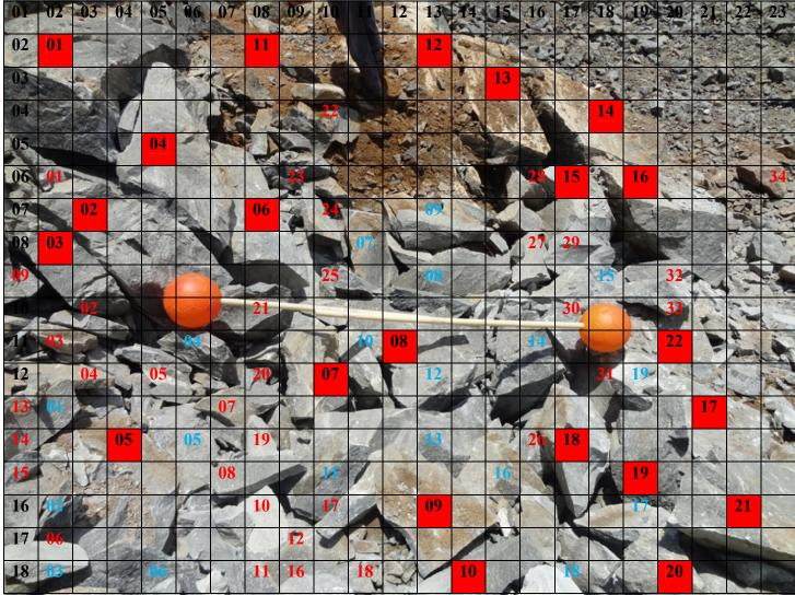
*Figure-17.4.1*: Location - 02, Blast -04 -Fragmentation Analysis (Scale : Ball diameter is 20.32 cm)
