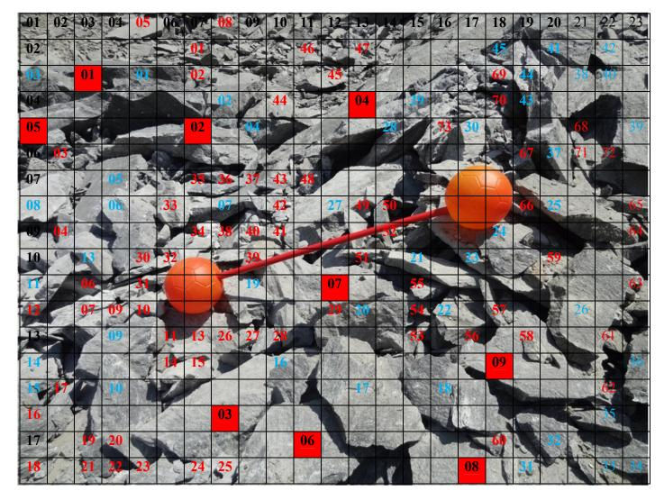
*Figure-19-1.1*: Location - 04, Blast -01-Fragmentation Analysis (Scale : Ball diameter is 20.32 cm)
