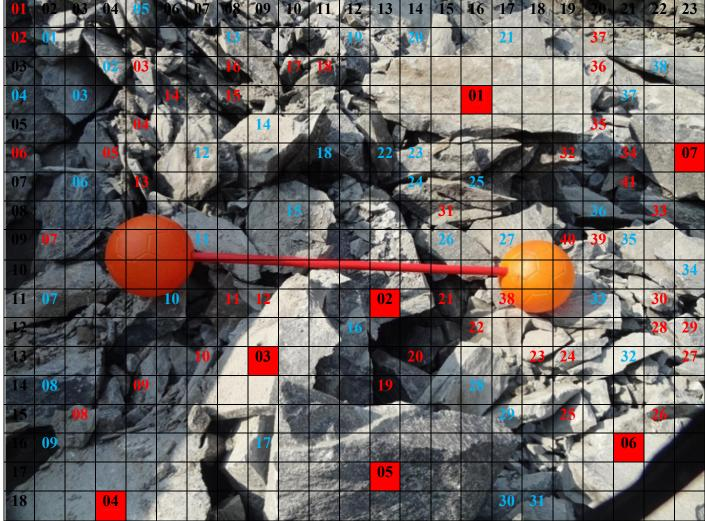
*Figure-19.2.1*: Location - 04, Blast -02 -Fragmentation Analysis (Scale : Ball diameter is 20.32 cm)
