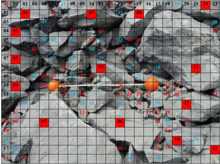
*Figure-20.1.1:* Location -05, Blast -01 -Fragmentation Analysis (Scale : Ball diameter is 20.32 cm)
