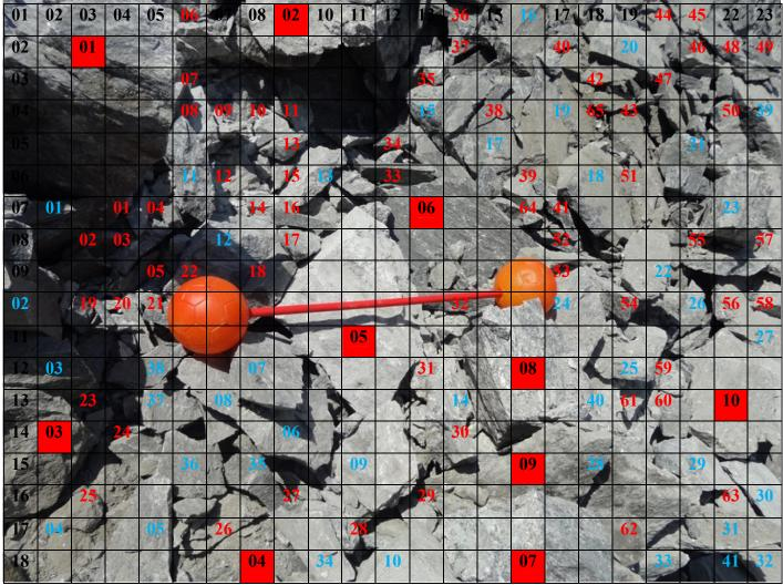
*Figure-19-4.1*: Location - 04, Blast -04 -Fragmentation Analysis (Scale : Ball diameter is 20.32 cm)
