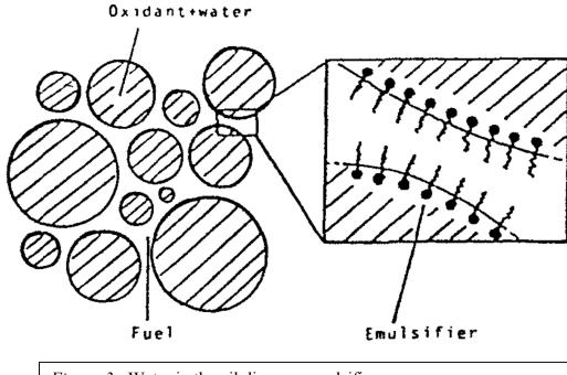
*Figure-3:* Water in the oil disperse emulsifier (Source - Internet – Ström,Tore et al - Ström&Gulliksson AB
