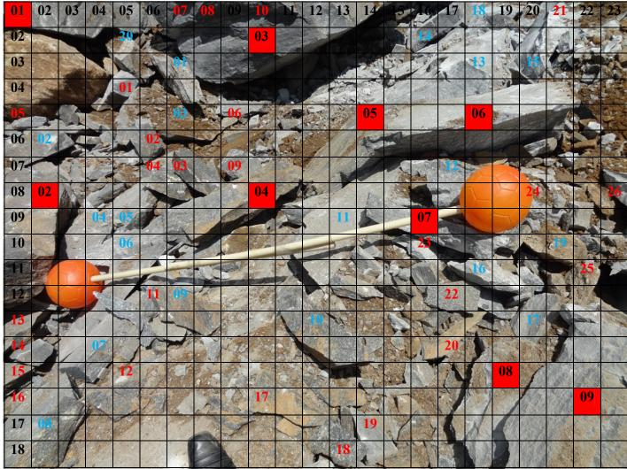
*Figure-17.6.1*: Location - 02, Blast -06 -Fragmentation Analysis (Scale : Ball diameter is 20.32 cm)
