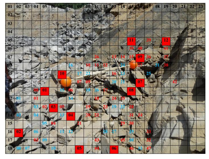
*Figure-18-2.1*: Location - 03, Blast -02 -Fragmentation Analysis (Scale : Ball diameter is 20.32 cm)
