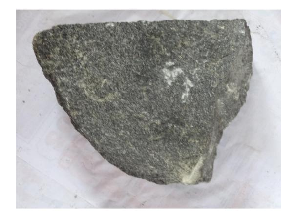
Figure-17: Rock Sample - Massive charnockite (fine grain) rock.
