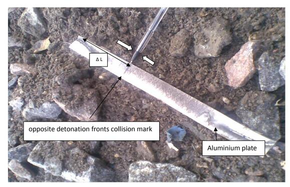
*Figure-7.2*: The distance from middle mark of detonating cord tocollision mark on the plate. ( $\Delta L$  = off centre distance of plate)
