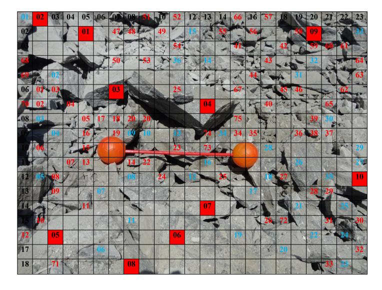
*Figure-19-6.1*: Location - 04, Blast -06 -Fragmentation Analysis (Scale : Ball diameter is 20.32 cm)
