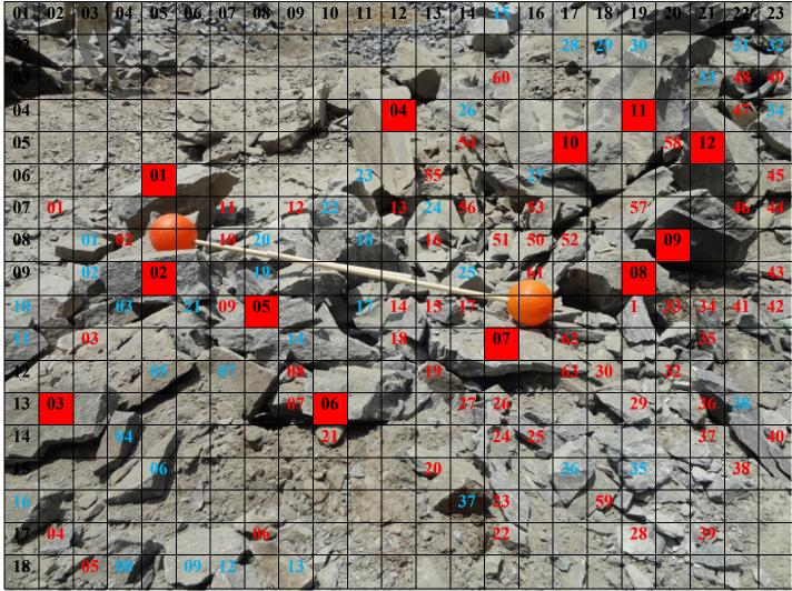
*Figure-18-4.1*: Location - 03, Blast -04 -Fragmentation Analysis (Scale : Ball diameter is 20.32 cm)
