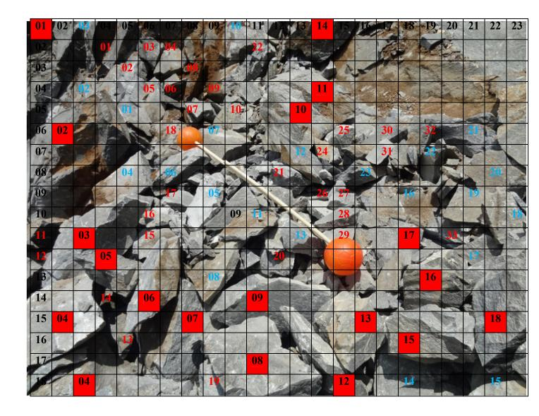
*Figure-17.3.1*: Location - 02, Blast -03-Fragmentation Analysis (Scale : Ball diameter is 20.32 cm)
