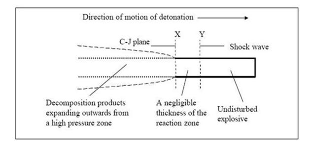
*Figure-1* . Sketch of detonation head. [Source– Internet:-Rock breakage and blast design considerations in open pit, by Dr. ParthaDasSharma.]
