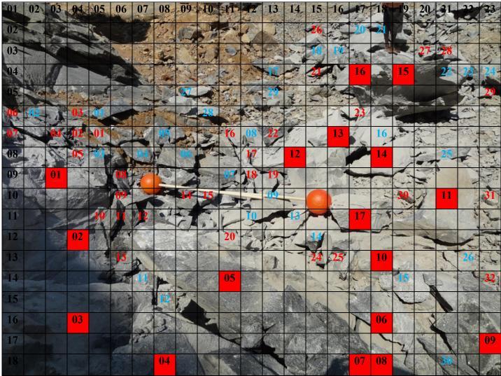
*Figure-18.1.1*: Location - 03, Blast -01 -Fragmentation Analysis (Scale : Ball diameter is 20.32 cm)
