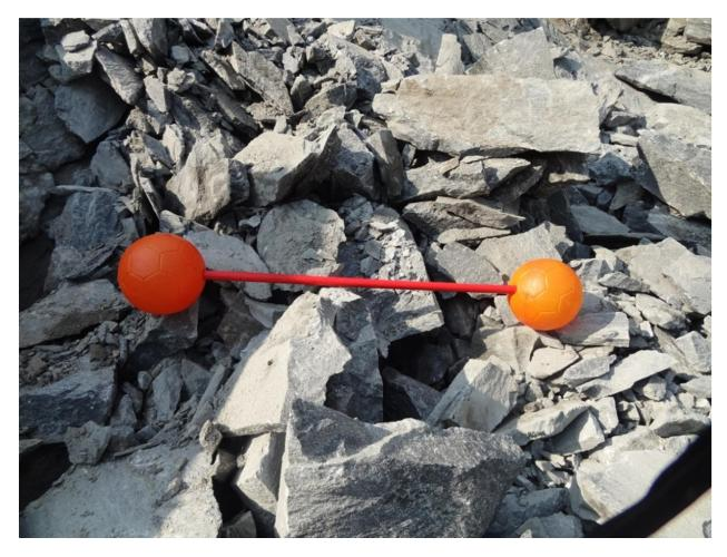
*Figure-19.2*: Location - 04,Blast -02- (Scale: Ball diameter is 20.32 cm)
