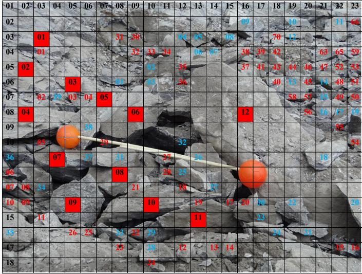
*Figure-21.1.1* :Location - 06, Blast -01-Fragmentation analysis (Scale : Ball diameter is 20.32 cm)
