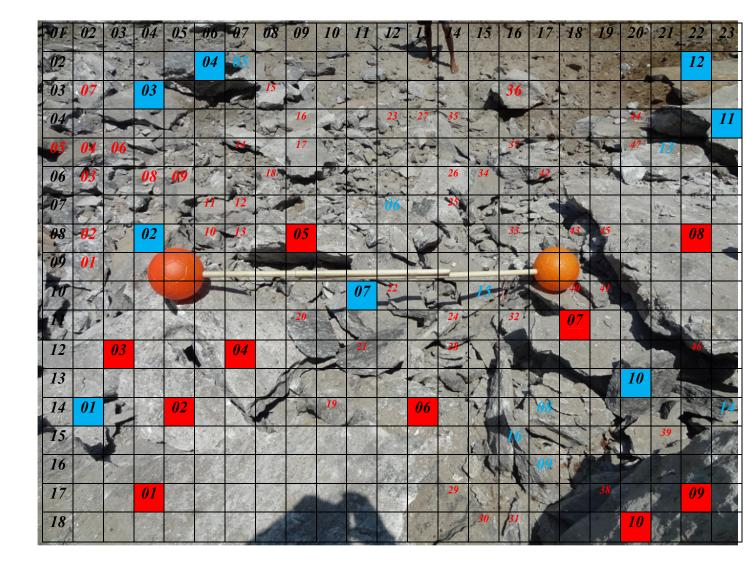
*Figure-16.3.1:* Location -01, Blast -03, Fragmentation Analysis -(Scale: Ball Diameter is 20.32cm)
