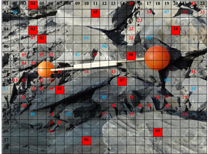
*Figure-16.4.1*: Location -01, Blast -04, Fragmentation Analysis - (Scale: Ball Diameter is 20.32cm)
