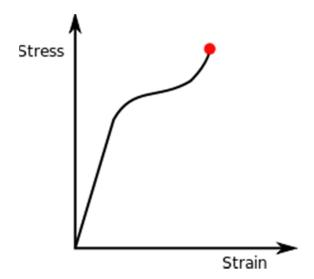
*Figure-10* : Typical stress-strain curve (Hook's law). Source - Internet
