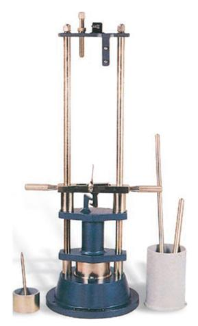
*Figure-8*: Aggregate impact tester [Source- http://www.enkaymachine.com/productsdetail.php?cat=Ng==&product= MjYy . Abrasion: Ref. standards IS:2386 part (4), BS:812, ASTM C-131, D2, AASHOT T96]
