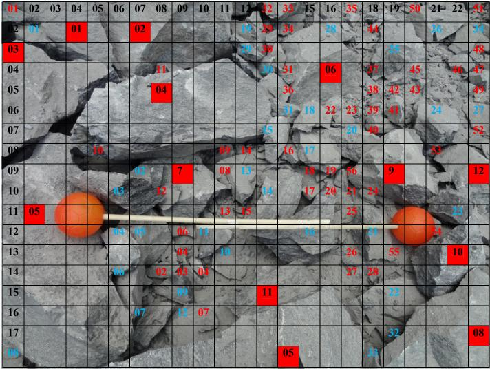
*Figure-20.6.1*: Location -05, Blast -06-Fragmentation Analysis (Scale : Ball diameter is 20.32 cm)
