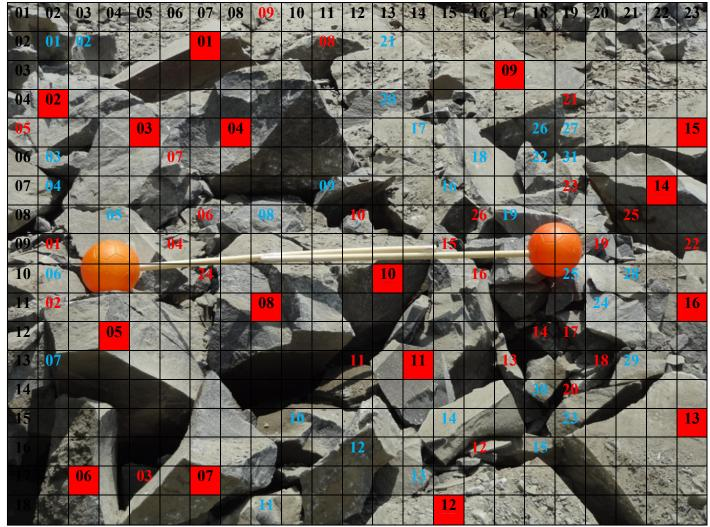
*Figure-18-3.1*: Location - 03, Blast -03 -Fragmentation Analysis (Scale : Ball diameter is 20.32 cm)
