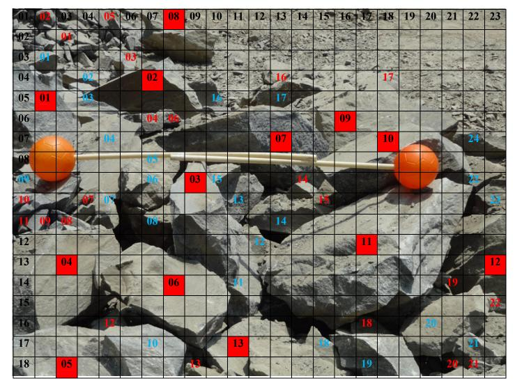
*Figure-18-6.1*: Location - 03, Blast -06 -Fragmentation Analysis (scale : Ball diameter is 20.32 cm)
