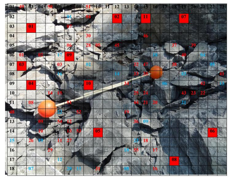
*Figure-16.2.1*: Location -01, Blast -02, Fragmentation Analysis -(Scale - Ball diameter is 20.32cm)
