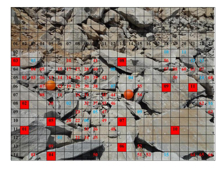
*Figure-16.5.1* :Location -01, Blast -05, Fragmentation Analysis - (Scale: Ball Diameter is 20.32cm)
