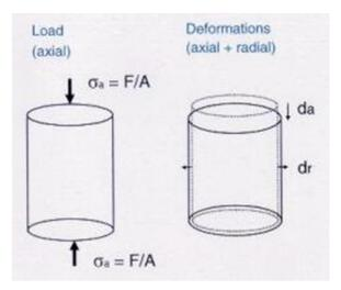
*Figure-9* : Applied loads with materials deformations Source - internet.
