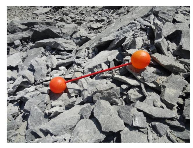
Figure-19.1 :location - 04, Blast -01 - (Scale: Ball diameter is 20.32 cm)
