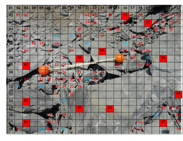
*Figure-16.6.1*: Location -01, Blast - 06, Fragmentation Analysis -(Scale: Ball diameter is 20.32cm)
