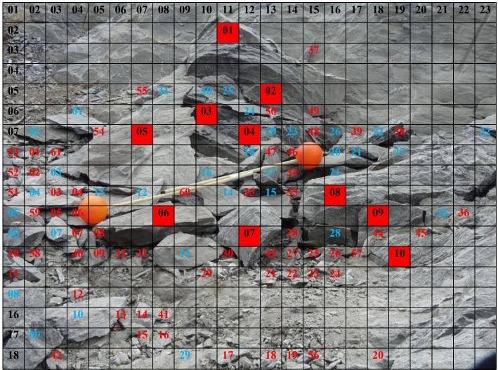
*Figure-21.5.1*: Location - 06, Blast -05, Fragmentation analysis (Scale : Ball diameter is 20.32 cm)
