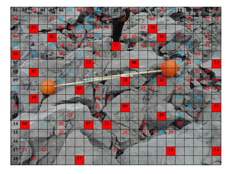
*Figure-20-4.1*: Location -05, Blast -04 -Fragmentation Analysis (Scale : Ball diameter is 20.32 cm)
