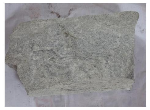
*figure-16*:Rock Sample, Quartz feldspar fine grain, light colour biotite rock with banding (leucocratic rock).
