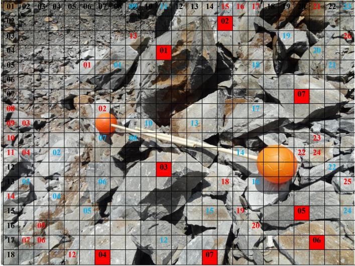
*Figure-17.5.1*: Location - 02, Blast -05 -Fragmentation Analysis (Scale : Ball diameter is 20.32 cm)
