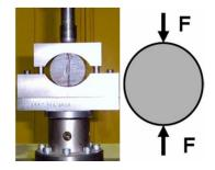
*Figure-14* : Load applied for indirect tensile strength test. Source - Internet
