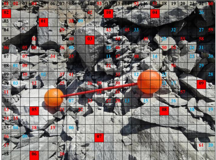
*Figure-19-3.1*: Location - 04, Blast -03 -Fragmentation Analysis (Scale : Ball diameter is 20.32 cm)
