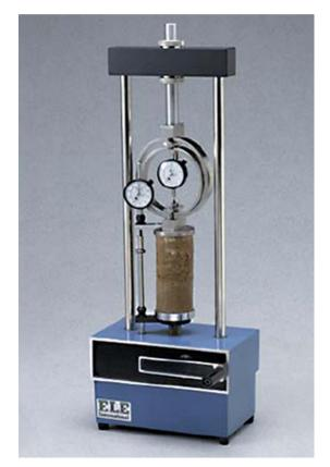
*Figure-12*: Uniaxial unconfined compression tester. [Source - internet - http://www.enkaymachine.com/products detail.php?cat=Mg==&product=MTAw]
