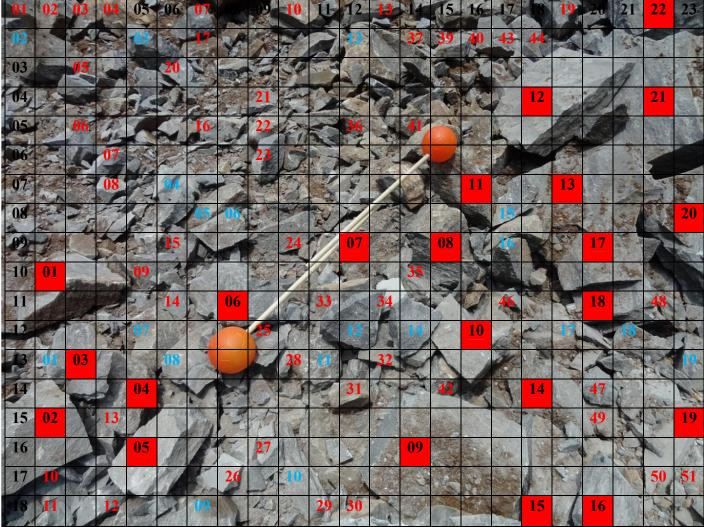
*Figure-17.1.1*: Location - 02, Blast -01 -Fragmentation Analysis (Scale : Ball diameter is 20.32 cm)
