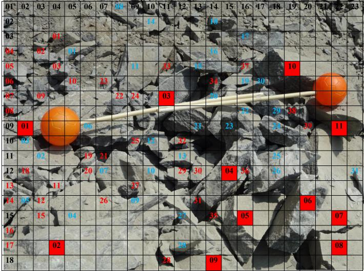
*Figure-18-5.1*: Location - 03, Blast -05 -Fragmentation Analysis (Scale : Ball diameter is 20.32 cm)
