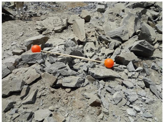
Figure-18-4 : Location - 03, Blast -04 - (Scale: Ball diameter is 20.32 cm)
