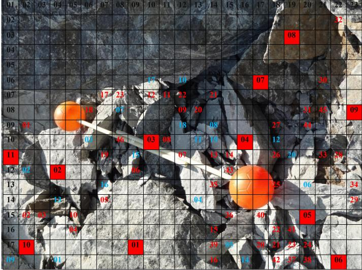
*Figure-16.1.1*: Location -01, Blast- 01, Fragmentation Analysis - (Scale - Ball diameter is 20.32cm)
