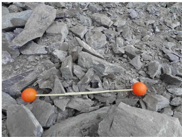
Figure-21.2: Location - 06, Blast -02- (Scale: Ball diameter is 20.32 cm)
