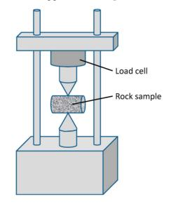
*Figure-13* : Point load test Source - Internet
