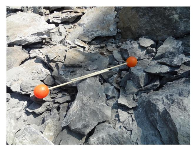
Figure-16.2: Location -01, Blast -02 - (Scale: Ball Diameter is 20.32cm)
