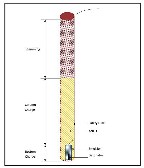
Figure - 5. Blast hole charging method
