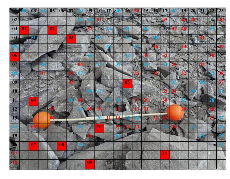
*Figure-21.2.1*: Location - 06, Blast -02 -Fragmentation analysis (Scale : Ball diameter is 20.32 cm)
