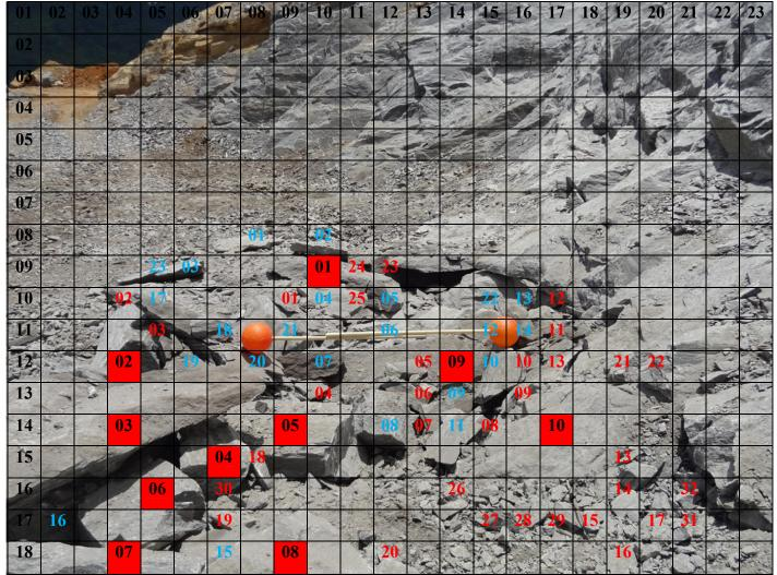
*Figure-21.6.1*: Location - 06, Blast -06, Fragmentation analysis (Scale : Ball diameter is 20.32 cm)
