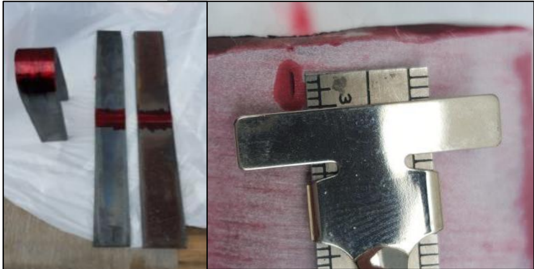
Application of the penetrant After applying the developer to aid in the discovery of cracks
