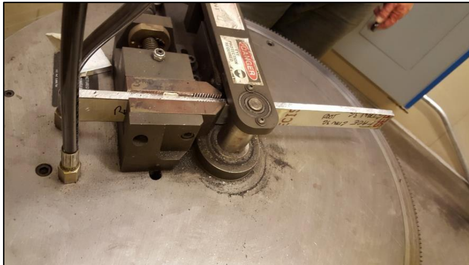
Figure 6.3 -The mechanical wraparound bend test measures the ductility of a weld[7]
