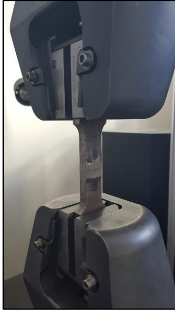
Figure 6.4 -The reduced section tensile test measured the tensile strength of a welded sample[7]
