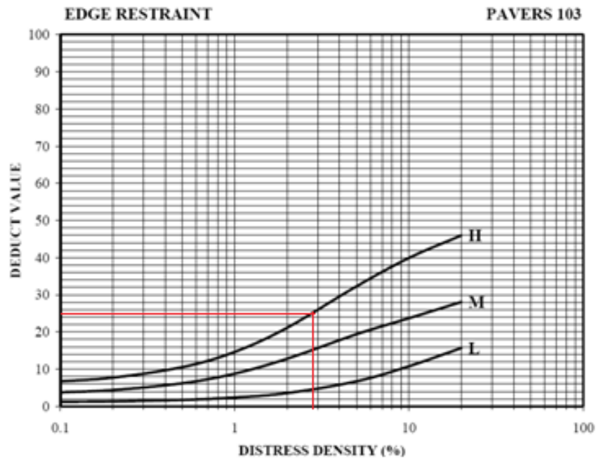
Figure 3-7 Deduct curves for edge restrain
