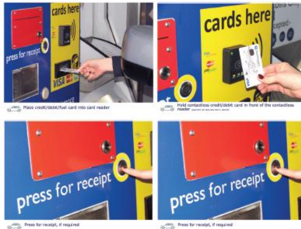
Figure 43: Facility for use of Credit cards/ prepaid contact less cards for toll payments
