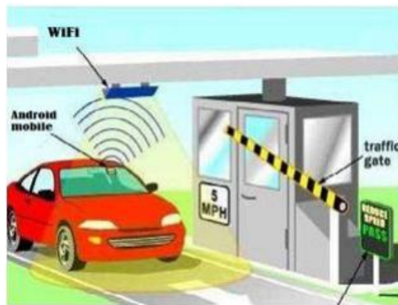
Figure 20: System layout at toll booth using Wi-Fi
