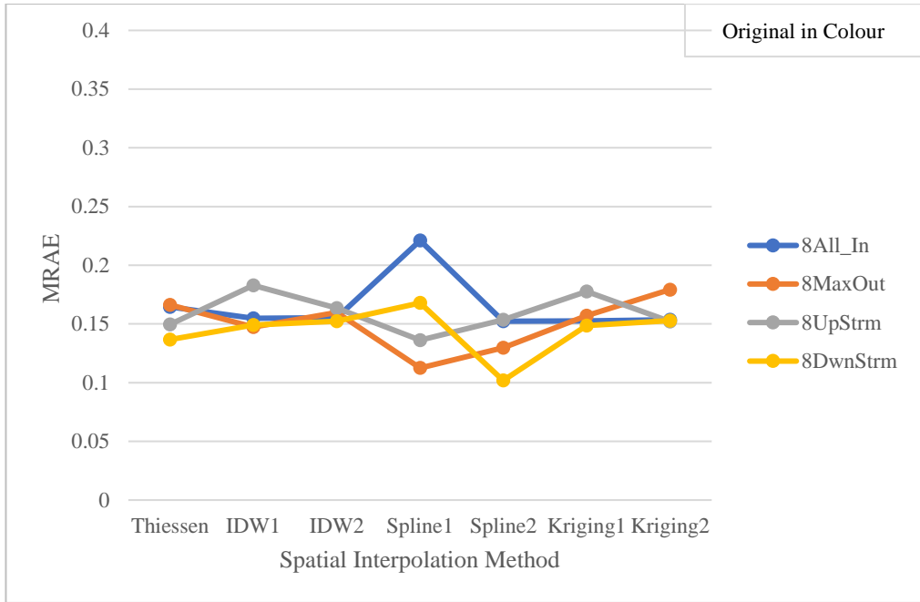
Figure 6-18: Flow Duration Curve fitting MRAE variation for different 8 stations configurations
