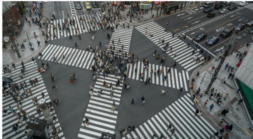
Plate 4.7.2.1 - an exclusive pedestrian phase of a junction
