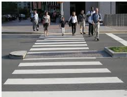
Figure 2.06: Pedestrians on a Zebra crossing with an island (Source: https://metro.co.uk )
