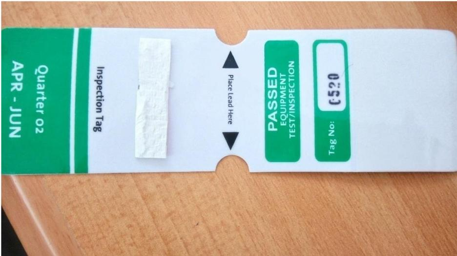
Figure 7.8 Equipment test tag
