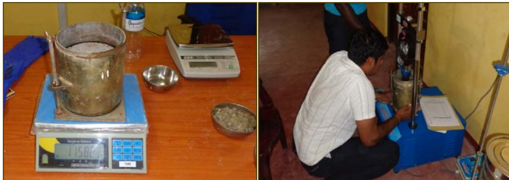
Figure 4.5: CBR sample measures and testing
